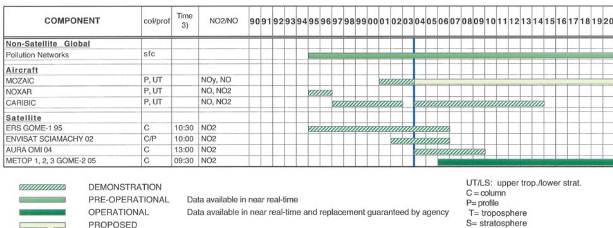
Figure 4.10. An overview of satellite, ground-based and aircraft measurements for tropospheric NO_2 .
