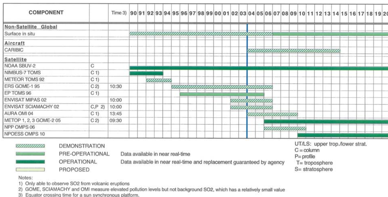
Figure 4.13. An overview of satellite, ground-based and aircraft measurements for SO 2 .
